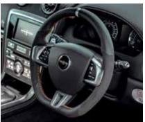
Contoured, flat-bottomed Alcantara® and leather-trimmed, with contrast tan stitching finished with a brushed aluminium centre-marker. Machined aluminium gear selectors are mounted
